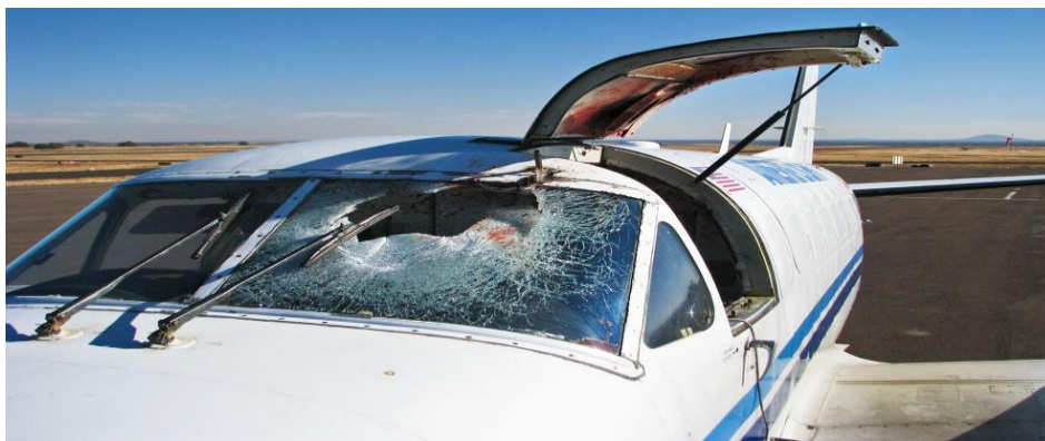
Plate 5: A Windscreen of an aircraft that was hit by a bird Source: http://www.birdstrikenews.com . Accessed April 2014
